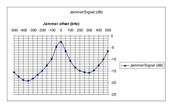
Disregarding the data points at  $-450~\rm kHz$ ,  $-400~\rm kHz$ ,  $-350~\rm kHz$ , and  $-300~\rm kHz$ , the worst data point is found to be at  $-16.6~\rm dB$  (at  $-250~\rm kHz$ ). Thus, the PG becomes
