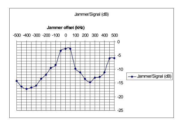
Disregarding the data points at  $-450~\rm kHz$ ,  $-400~\rm kHz$ ,  $-350~\rm kHz$ , and  $-300~\rm kHz$ , the worst data point is found to be at  $-14.7~\rm dB$  (at  $+250~\rm kHz$ ). Thus, the PG becomes
