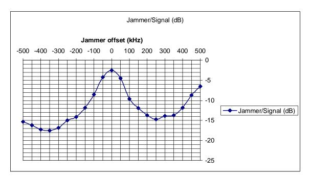
Disregarding the data points at -450 kHz, -400 kHz, -350 kHz, and -300 kHz, the worst data point is found to be at -15.3 dB (at -500 kHz). Thus, the PG becomes
