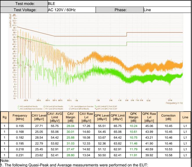
2. Margin[dB] = Limit[dB $\mu$ V] - Level[dB $\mu$ V]
