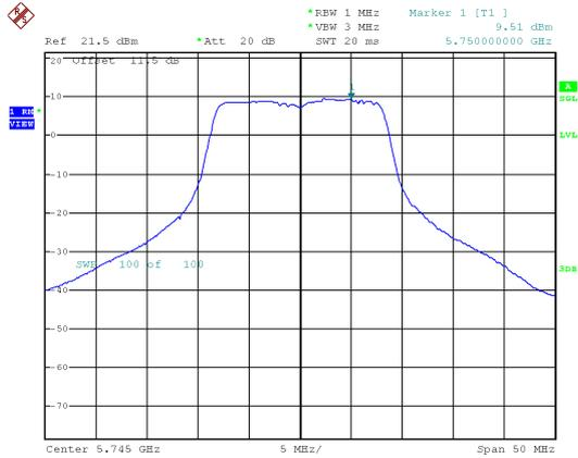
Modulation Standard: 802.11ac, VHT20 (6.5Mbps)
