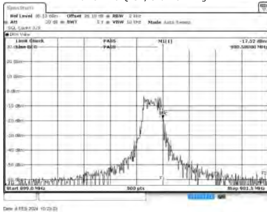
NB-IoT eFDD8 QPSK, Channel = high
