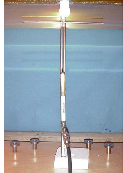
450MHz Dipole Setup
