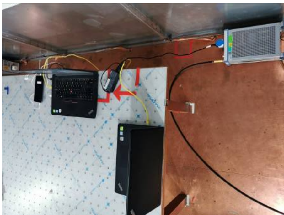
Conducted Emissions Test Setup (with laptop)
