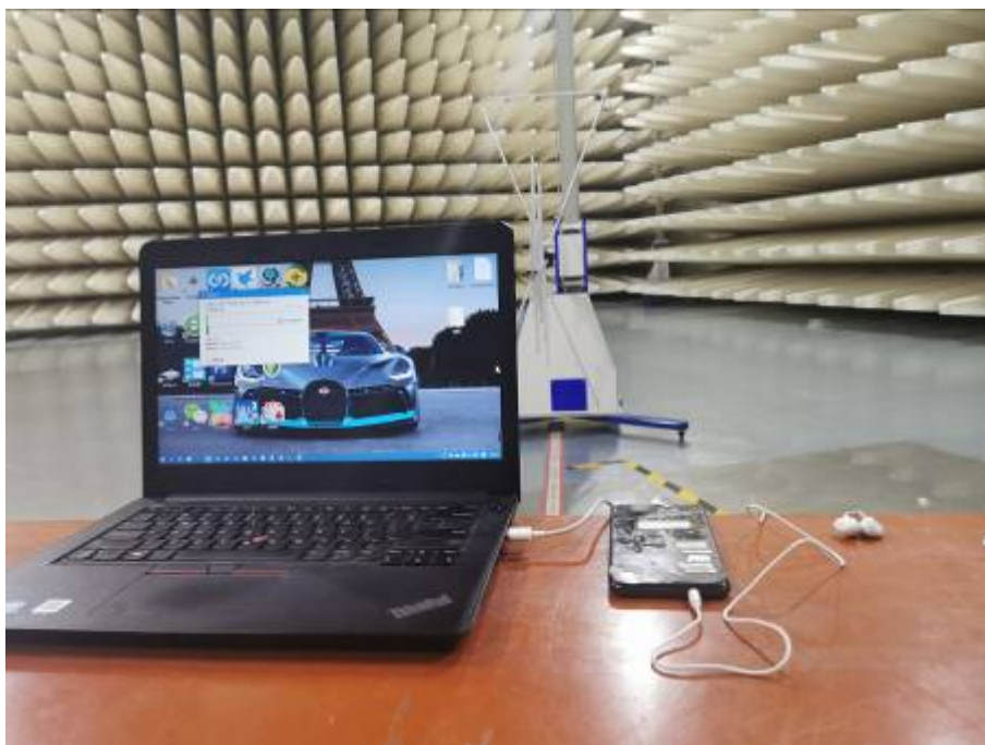
Radiated Emissions Test Setup (with laptop) (30-1000MHz)
