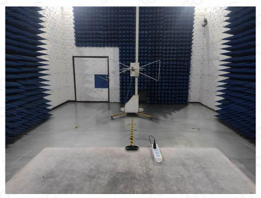
RADIATED EMISSION TEST SETUP ABOVE 1GHz
