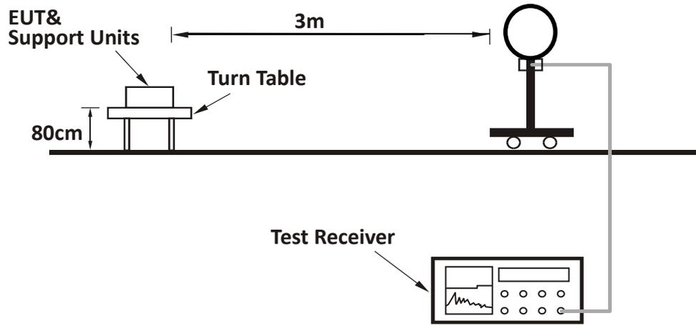
For Radiated emission 30MHz to 1GHz:
