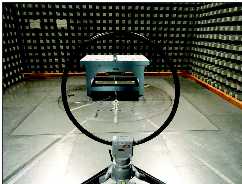
Photo 3: Radiated Test Sample-9 kHz to 30 MHz EUT Standing
