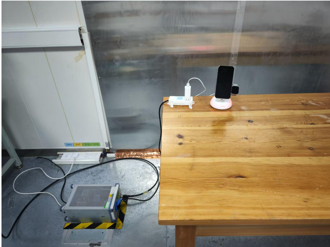
Conducted emission test setup
