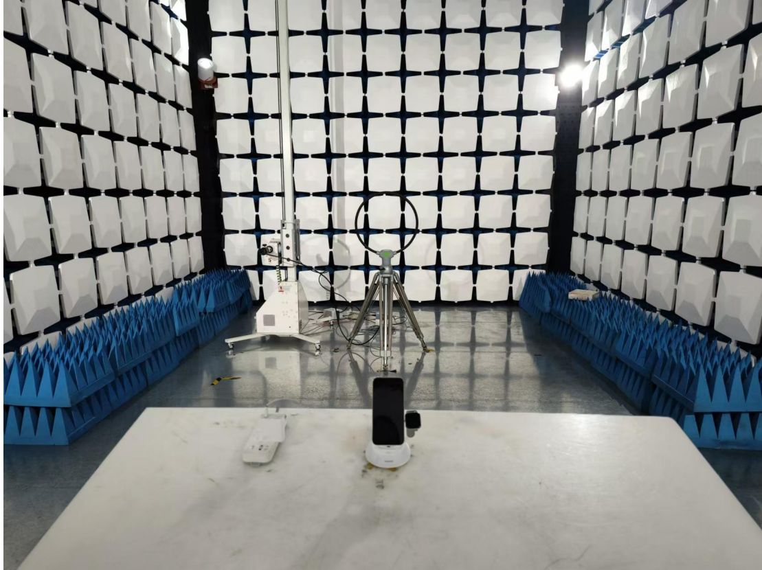
Blow 1GHz for radiated emission test setup
