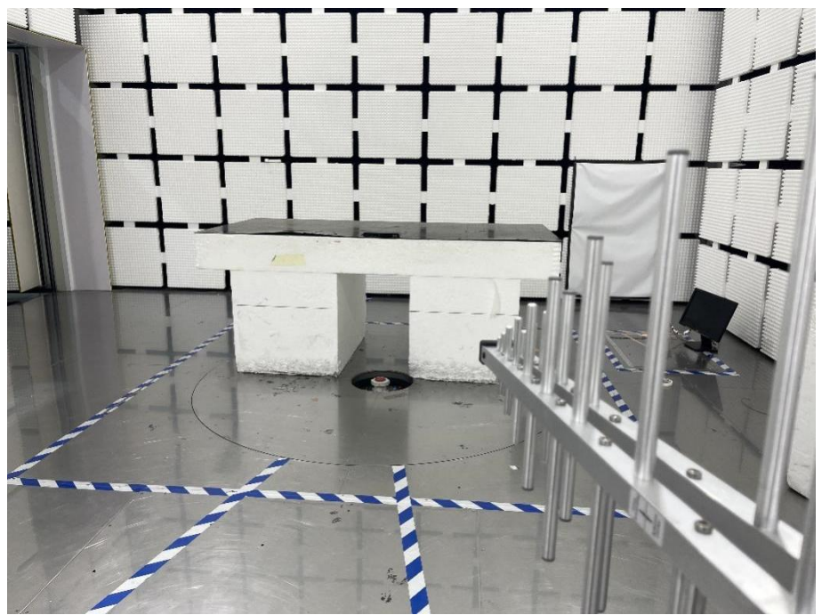
Radiation Emission Test Setup (30MHz to 1GHz)
