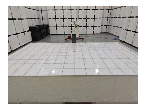
Set-up for Radiated Spurious Emission, Above 1GHz
