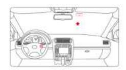
Tear off the 3M adhesive on the back of the remote control and take out the battery insulation sheet, and then stick the remote control on the steering wheel where it is easy to operate.
