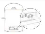
Plug the 6.5mm jack of the microphones to the Mic Aux-in ports
