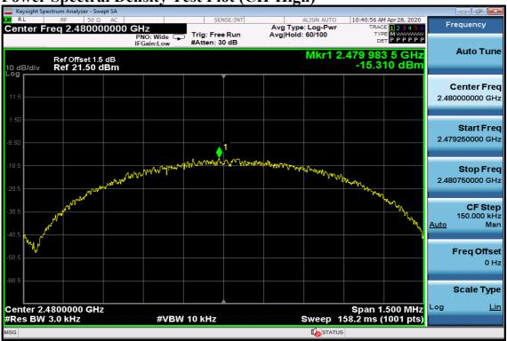
**BLE 4.2 Power Spectral Density Test Plot (CH-Low)**
