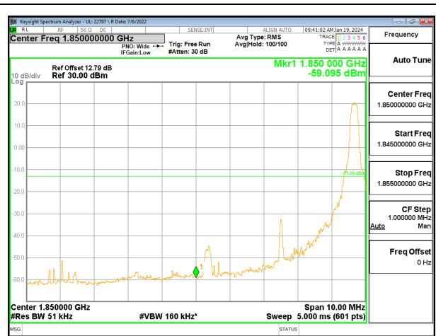
LTE Band 25 5MHz QPSK Low Channel RB1-24
