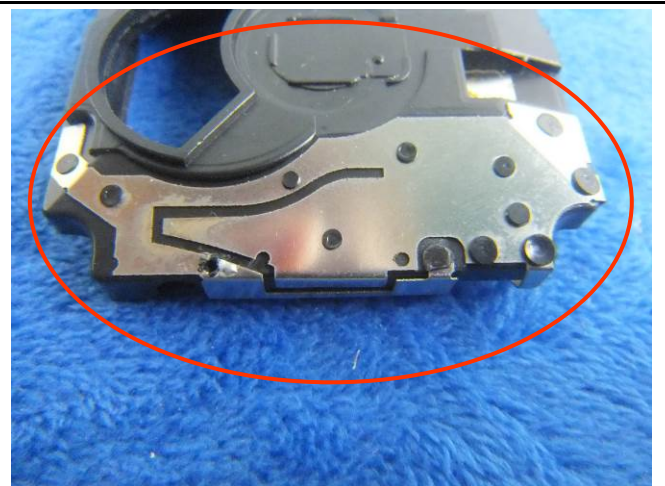
GSM/PCS Antenna View
