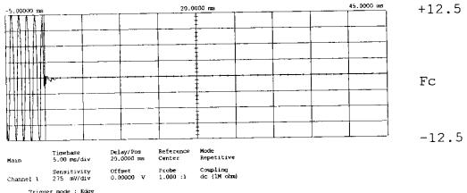
Trigger mode : Edge On Negative Edge Of Chan2 Trigger Level Chan2 = 31.500 mV (noise reject ON) Holdoff = 40.000 mS
