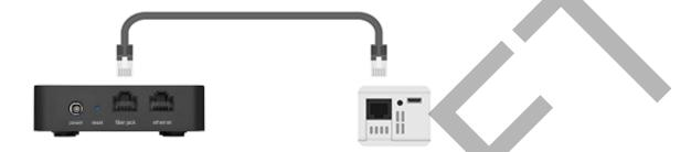
When the Mini Network Box is properly connected, the LED on the front lights up solid blue. If the LED does not light up solid blue about 2 minutes after being connected to power, contact Google Fiber customer support.
