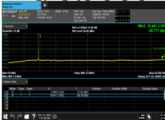
N77(25M)_DFT-s- OFDM QPSK Edge 1RB Left Mid CH
