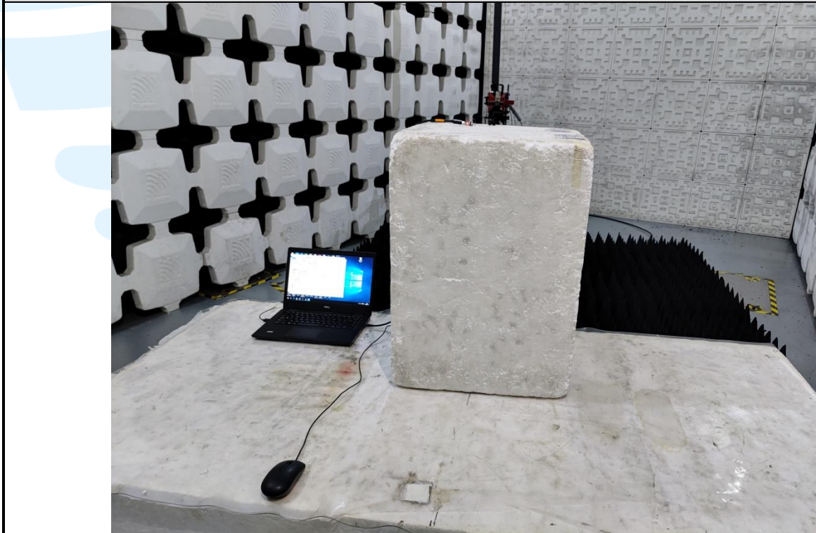
Radiated emission Test Setup (Above 1 GHz)
