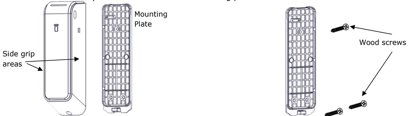
PRE-DRILL through the mounting plate at the three screw locations and INSERT wood screws.
