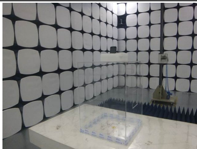
Radiated Spurious Emissions Test Setup Above 1GHz
