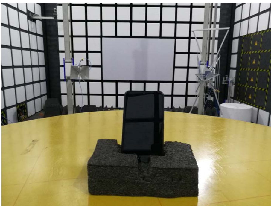
Spurious Radiated Emissions Test setup
