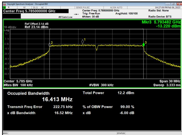
(802.11a) 6dB Bandwidth plot on channel 165
