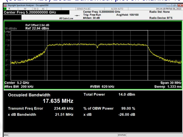
(802.11 n20) 26dB Bandwidth plot on channel 40
