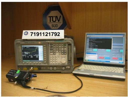
**Peak Power Spectral Density Test Setup**
