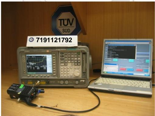
**RF Conducted Spurious Emissions Test Setup**
