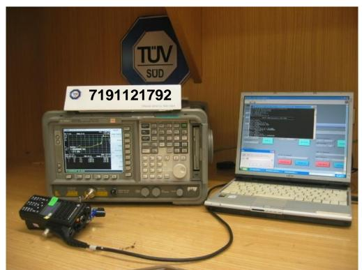
**Carrier Frequency Separation Test Setup**
