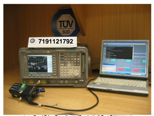
Band Edge Compliance (Conducted) Test Setup
