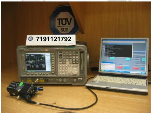
Spectrum Bandwidth (20dB Bandwidth Measurement) Test Setup
