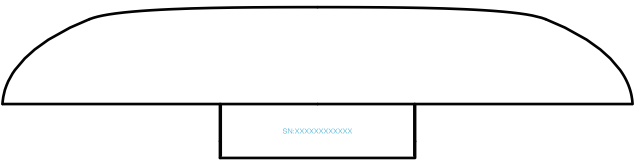
NS NUMBER top cover, hinge, interior face Laser etching Lighter color than background text height: 0.679 mm
