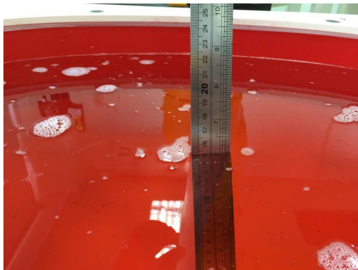
Photograph of the depth in the Head Phantom (450MHz)
