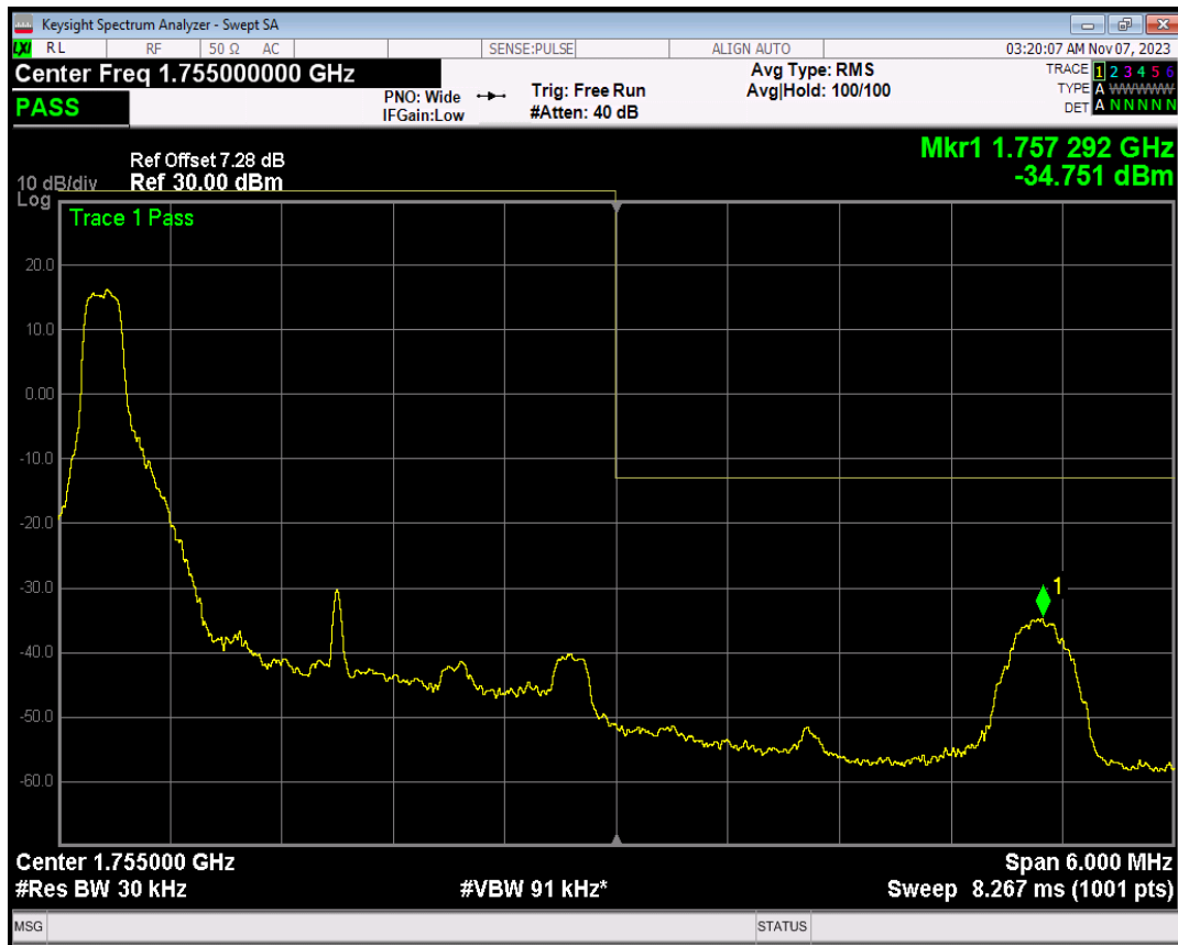
Band4 QPSK BW=3MHz Channel=20385 RB Size=1 Position=#Max
