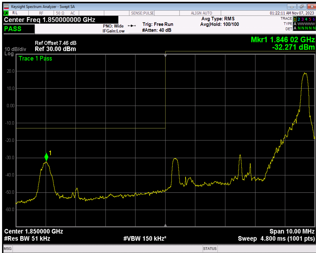
Band2 QPSK BW=5MHz Channel=18625 RB Size=25 Position=#0
