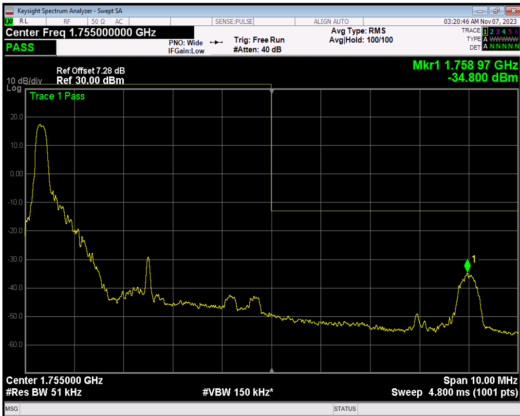
Band4 16QAM BW=5MHz Channel=20375 RB Size=1 Position=#Max
