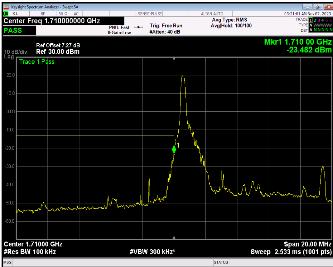
Band4 16QAM BW=10MHz Channel=20000 RB Size=1 Position=#Max
