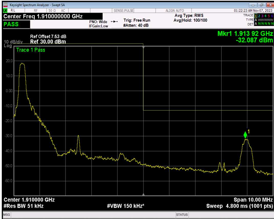
Band2 QPSK BW=5MHz Channel=19175 RB Size=1 Position=#Max
