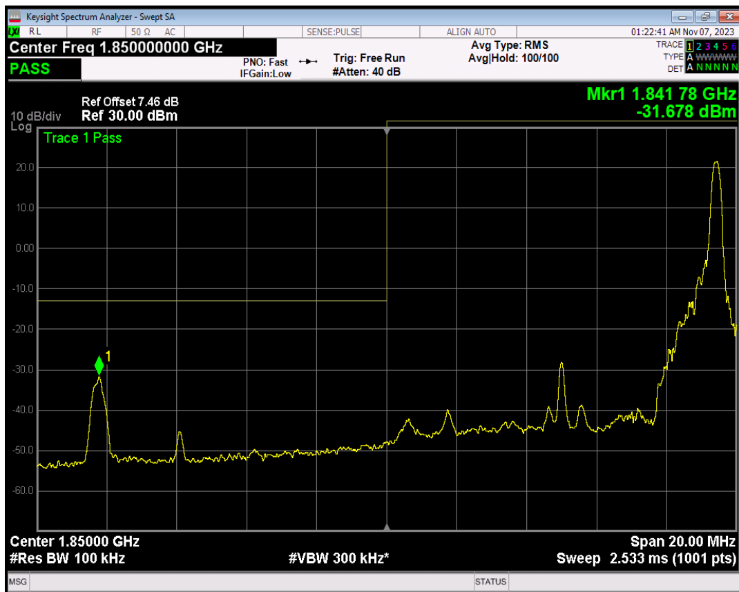
Band2 QPSK BW=10MHz Channel=18650 RB Size=50 Position=#0
