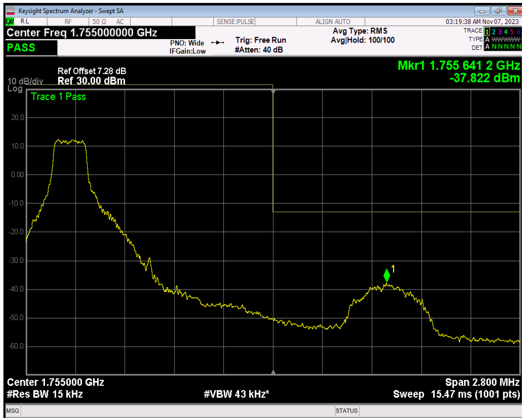
Band4 16QAM BW=1.4MHz Channel=20393 RB Size=1 Position=#Max
