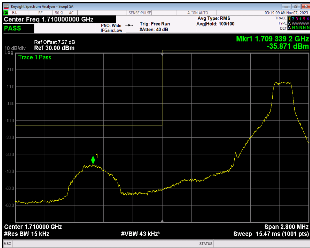
Band4 QPSK BW=1.4MHz Channel=19957 RB Size=6 Position=#0
