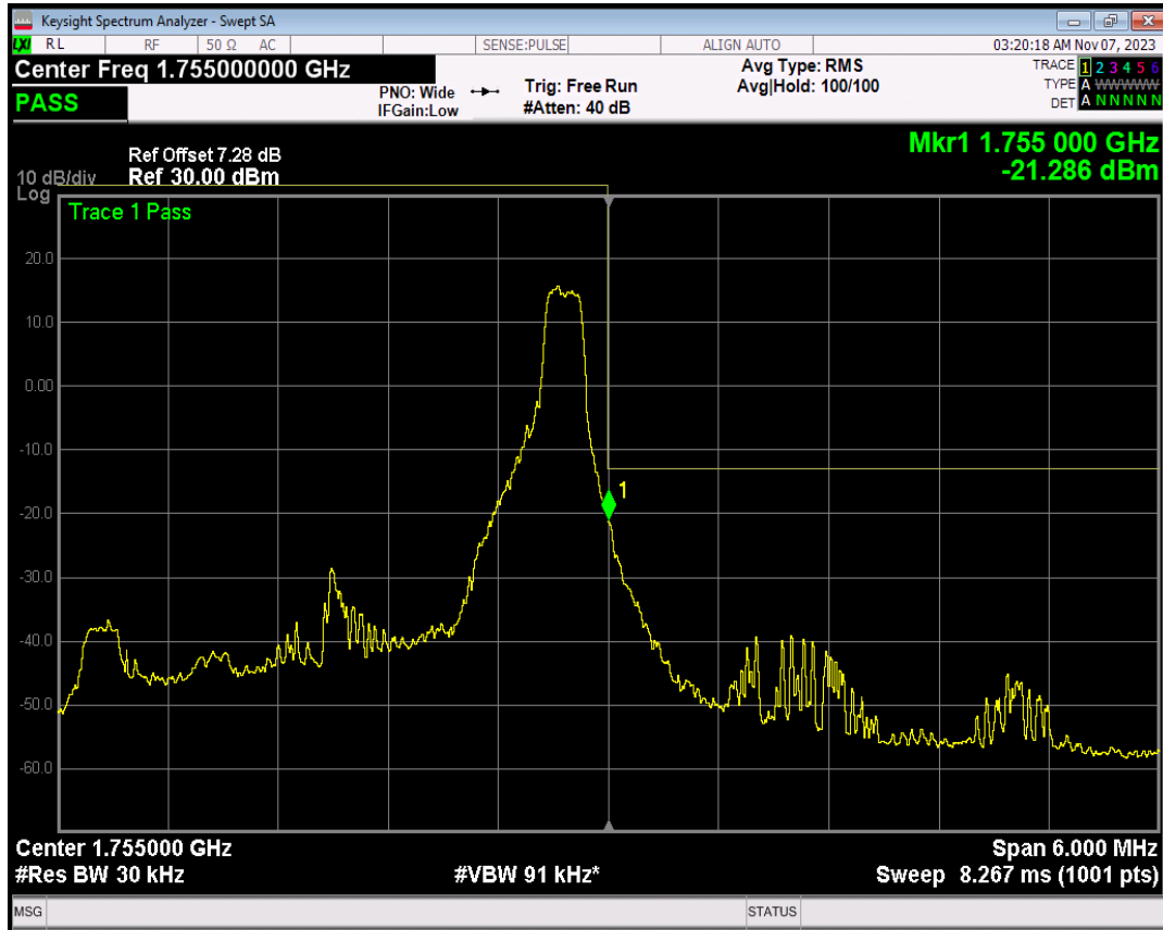
Band4 16QAM BW=3MHz Channel=20385 RB Size=15 Position=#0
