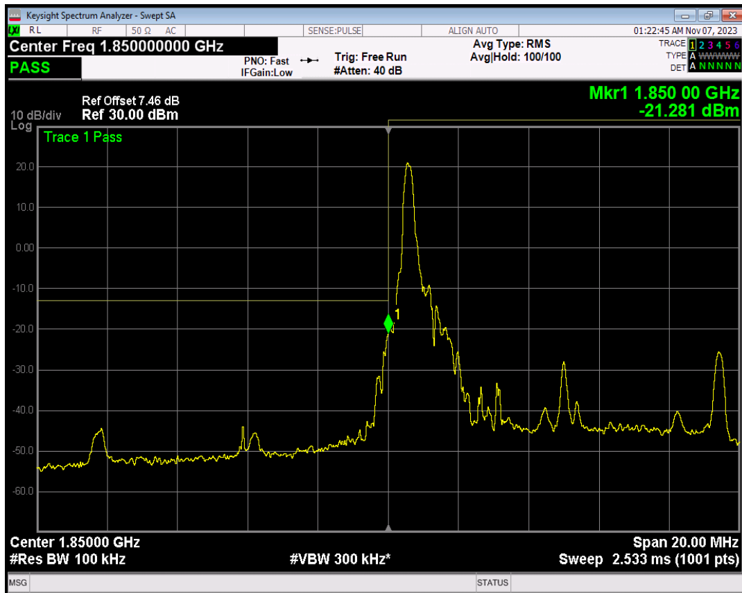
Band2 16QAM BW=10MHz Channel=18650 RB Size=1 Position=#Max
