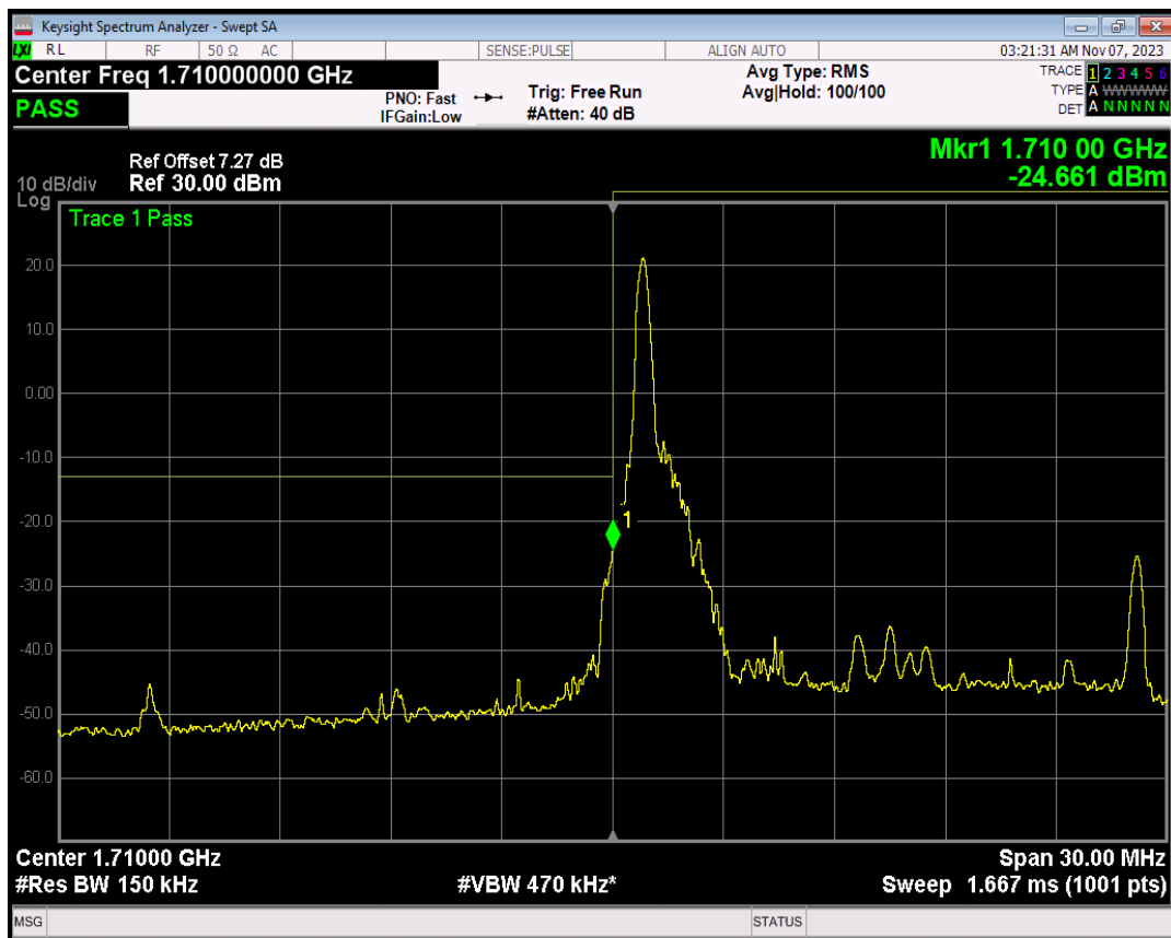
Band4 16QAM BW=15MHz Channel=20025 RB Size=1 Position=#Max
