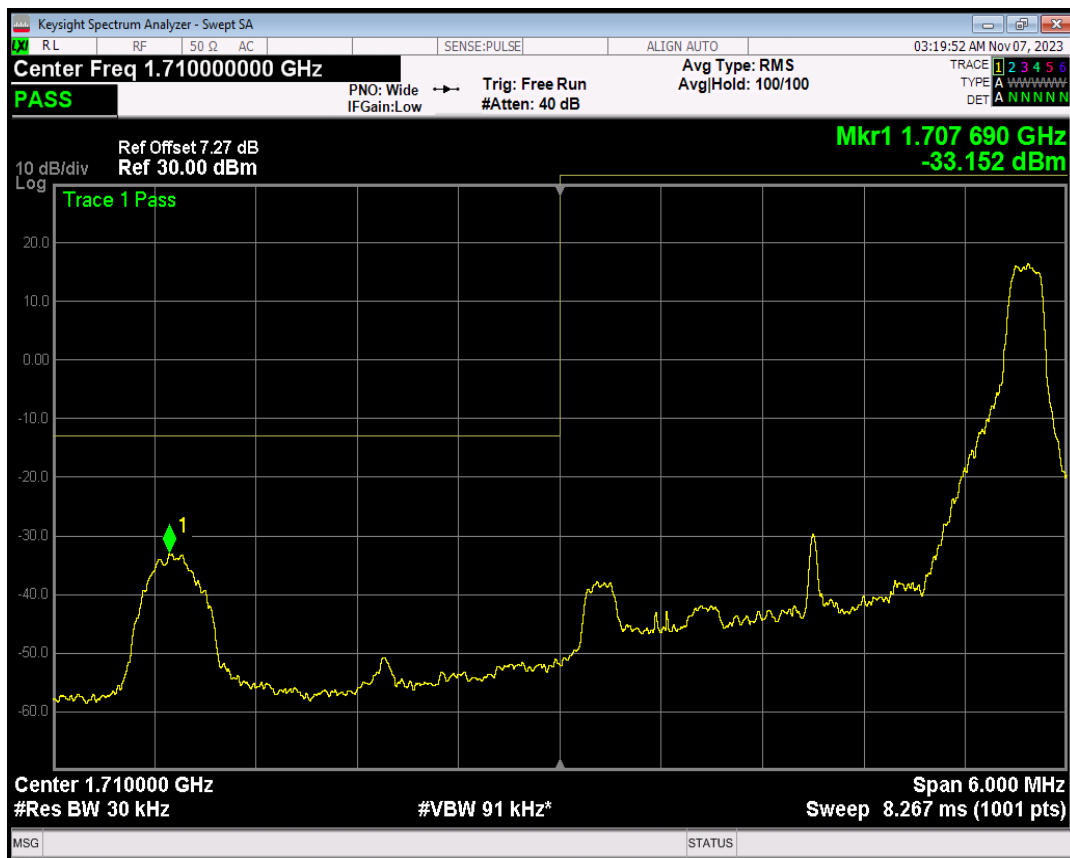
Band4 QPSK BW=3MHz Channel=19965 RB Size=15 Position=#0
