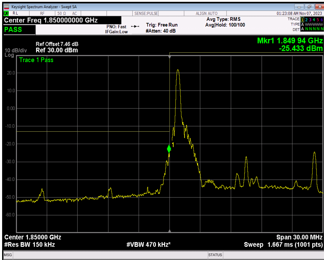
Band2 QPSK BW=15MHz Channel=18675 RB Size=1 Position=#Max
