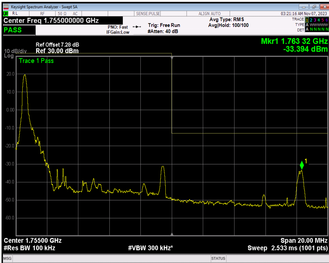
Band4 16QAM BW=10MHz Channel=20350 RB Size=1 Position=#Max
