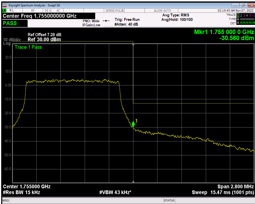
Band4 QPSK BW=3MHz Channel=19965 RB Size=1 Position=#0
