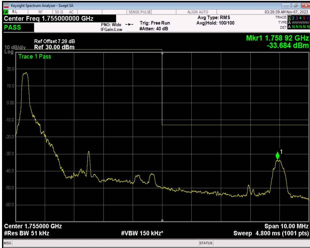
Band4 QPSK BW=5MHz Channel=20375 RB Size=1 Position=#Max
