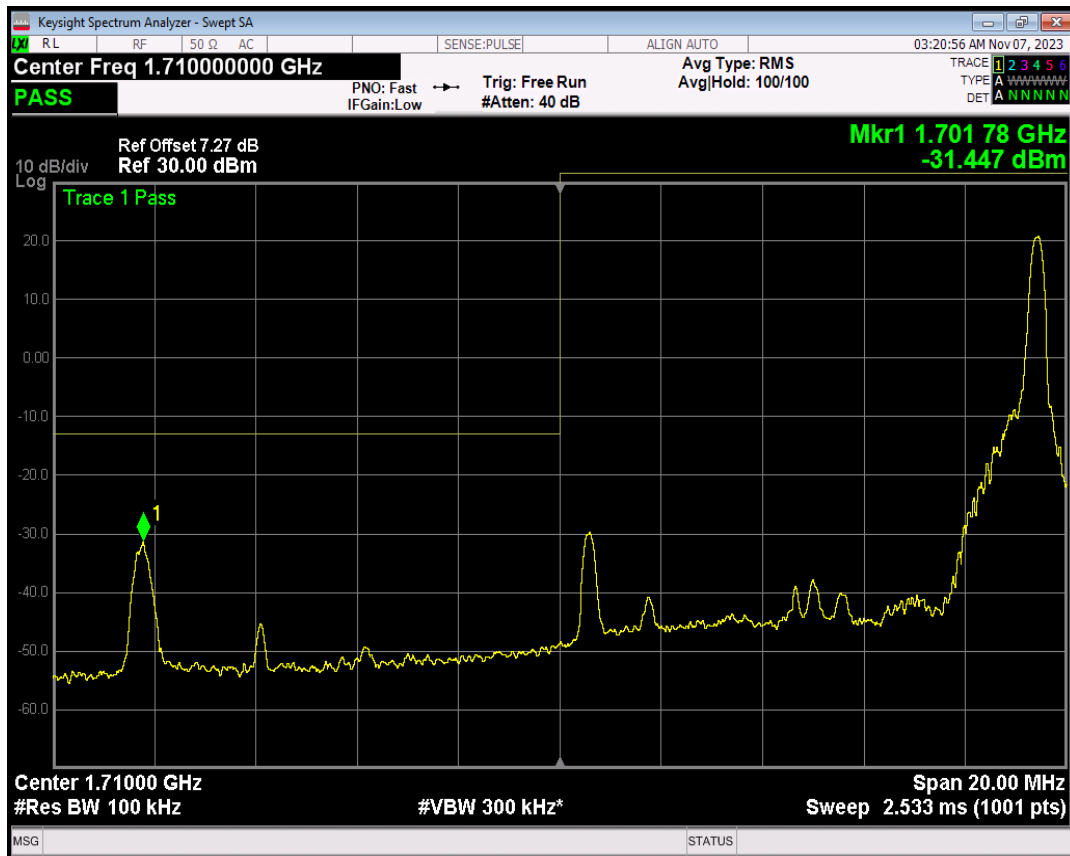
Band4 QPSK BW=10MHz Channel=20000 RB Size=50 Position=#0
