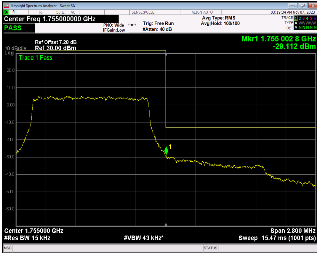
Band4 16QAM BW=1.4MHz Channel=20393 RB Size=1 Position=#0
