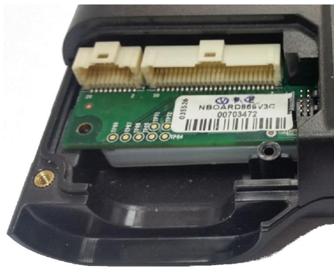
Figure 6: SmartHub OBC Interface connectors
