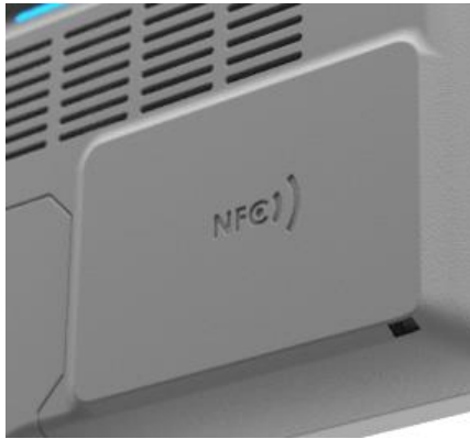
Figure 4: NFC Reader Antenna
