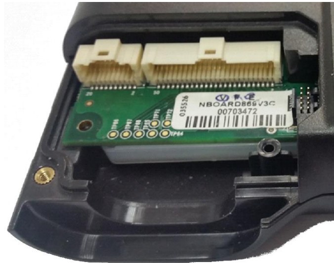
Figure 7: SmartHub OBC Interface connectors
