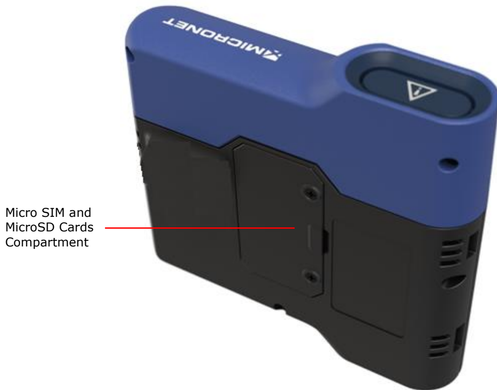
Figure 2: Micronet SmartHub Rear Panel View
