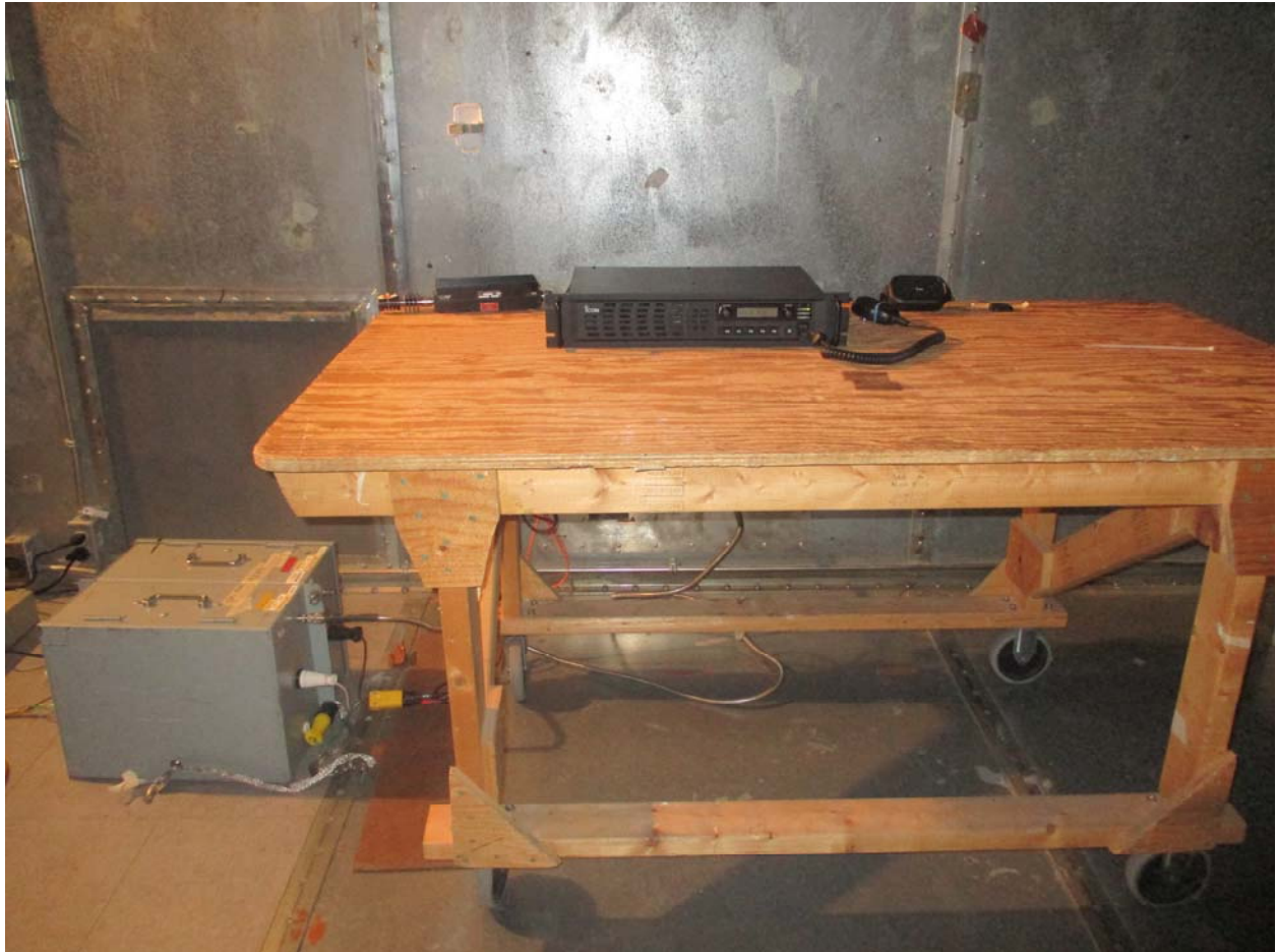
Power Line Conducted Setup
