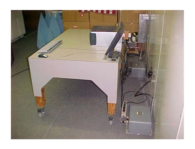
AC Conducted Emissions Measurement (Rear View) Setup
