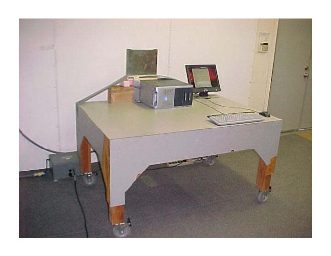
AC Conducted Emissions Measurement (Front View) Setup
