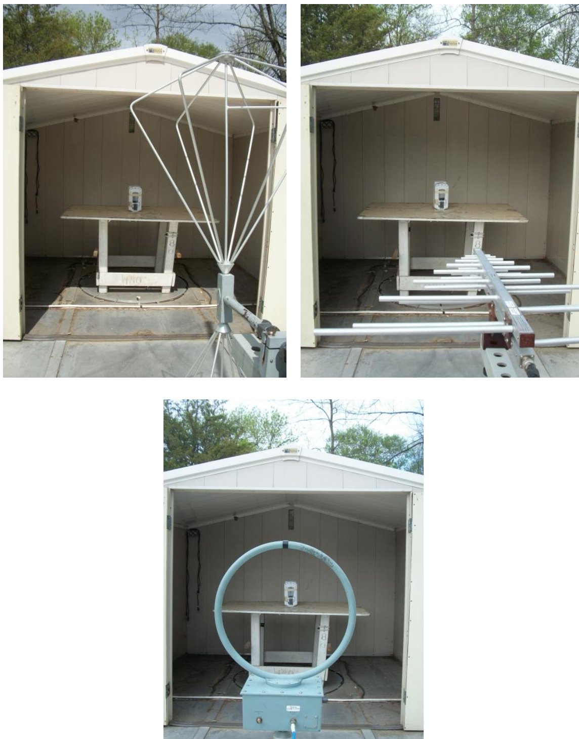
Figure 3.1 Radiated Test Setup
