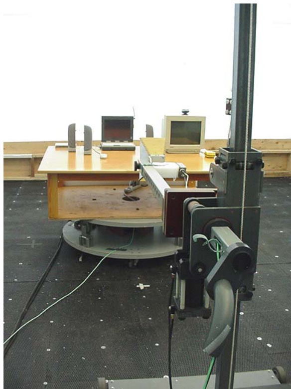
Photograph F.7-3 - Front of Radiated Emission Setup
