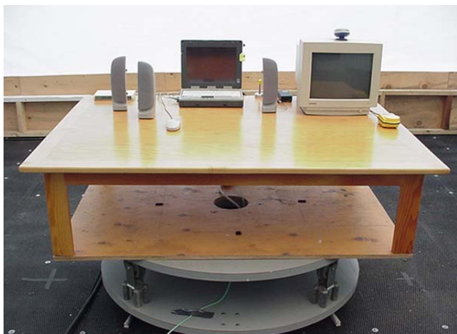
Photograph F.7-3 - Front of Radiated Emission Setup
