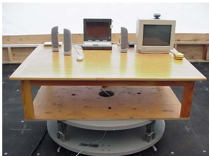
Photograph C.7-2 - Front of Radiated Emission Setup
