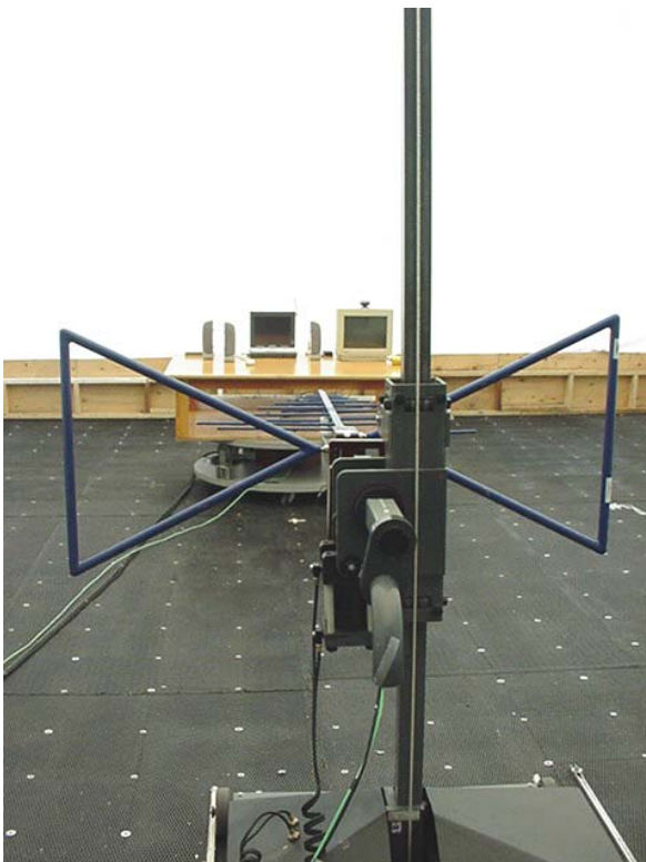
Photograph C.7-2 - Front of Radiated Emission Setup
