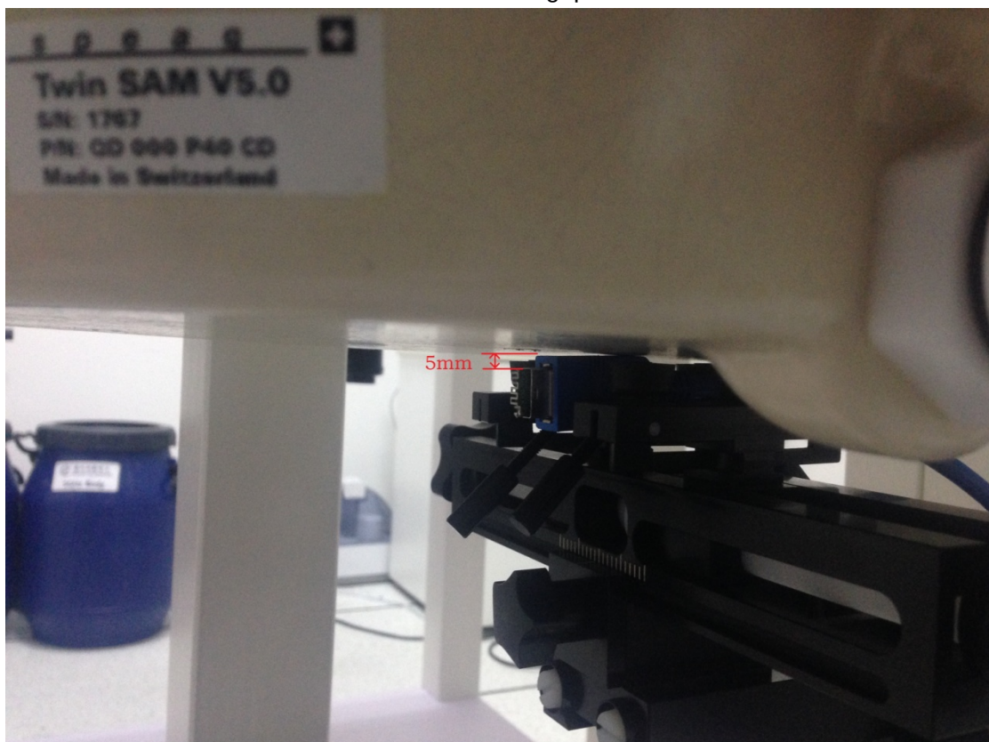
Vertical-Front view with gap 5mm
