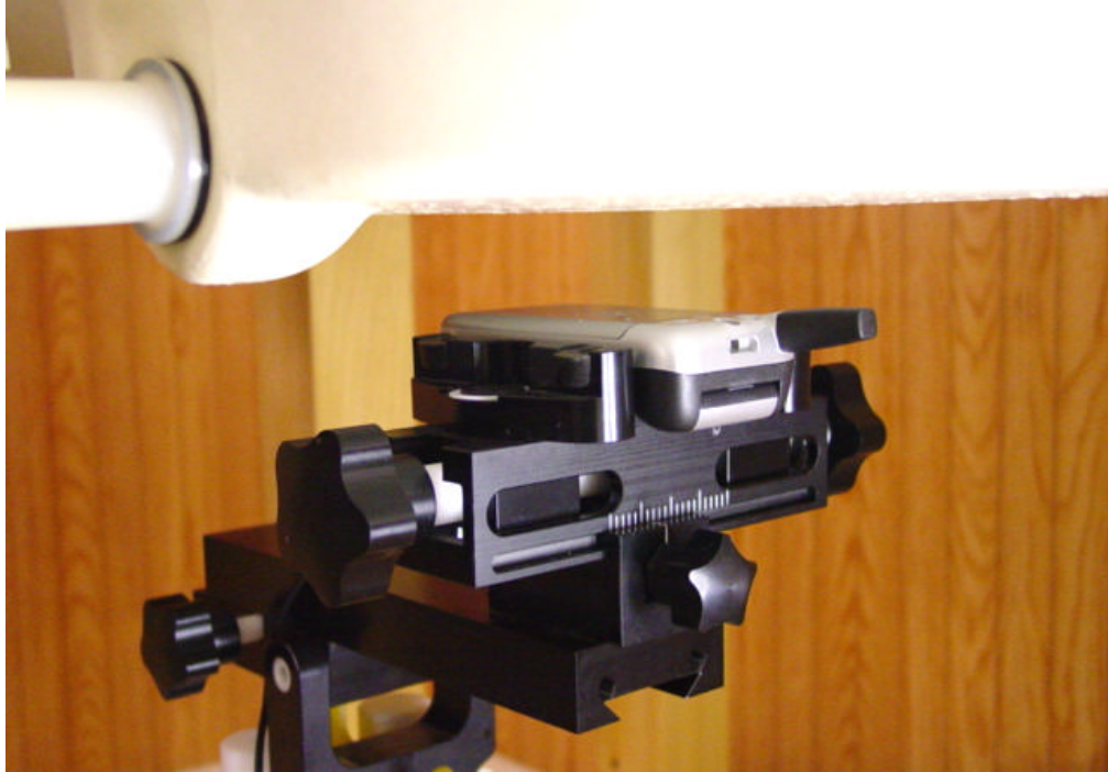
Figure 12.5 body SAR setup closed (with 25mm air separation)
