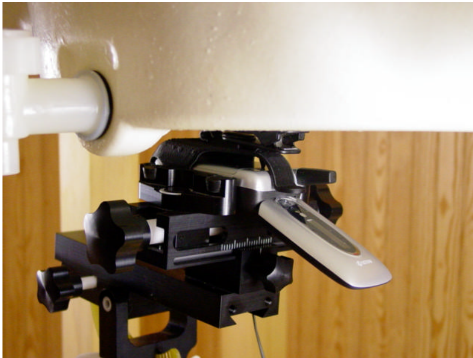
Figure 12.4 body SAR setup open (with holster)
