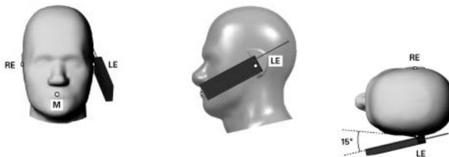
Figure 9.3 - Phone position 2, “tilted” position.
