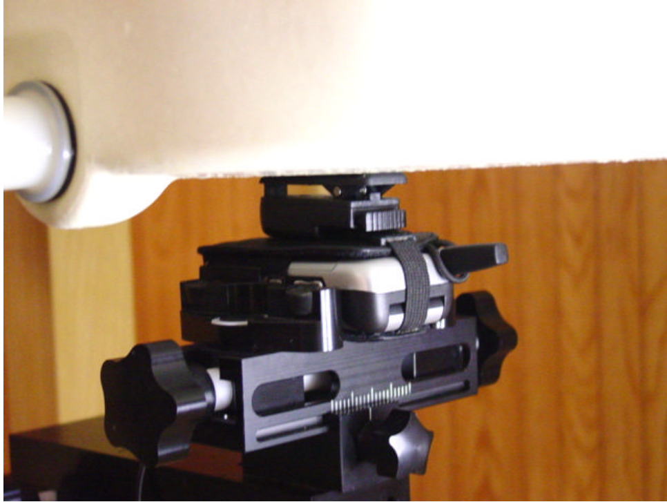
Figure 12.7 body SAR setup closed (with leather case)
