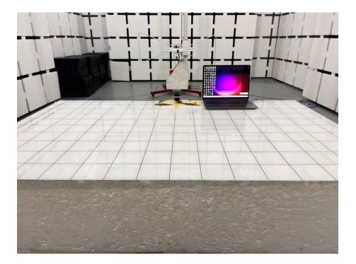
Set-up for Radiated Spurious Emission, Below 1GHz
