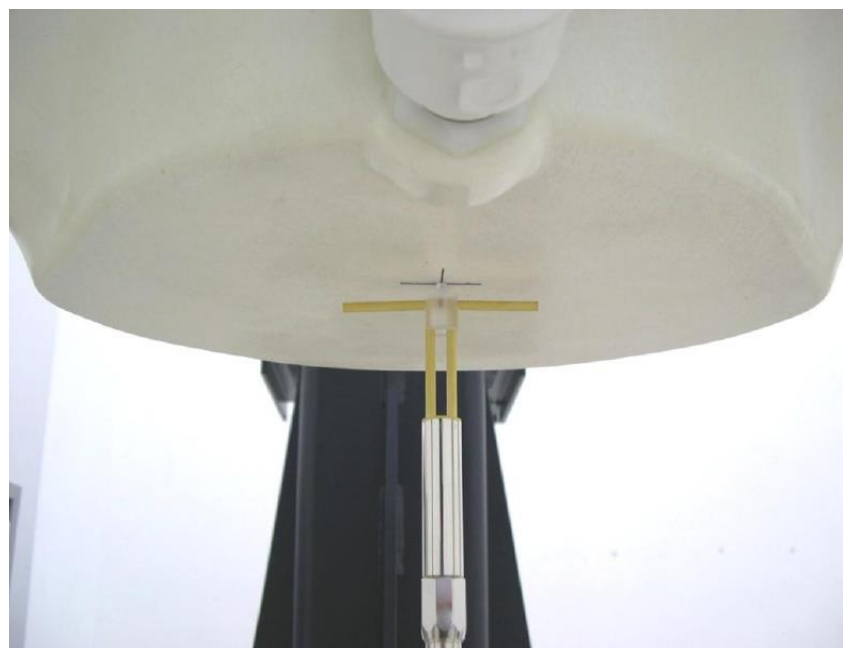
Picture 8.2 Photo of Dipole Setup
