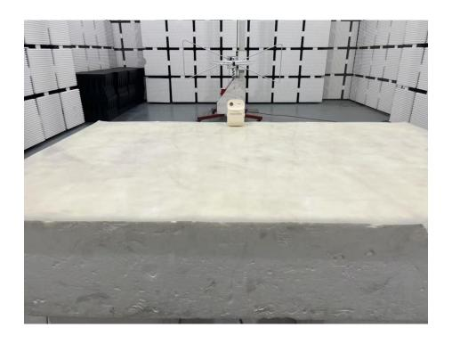
**Set-up for Radiated Spurious Emission, Above 1GHz**
