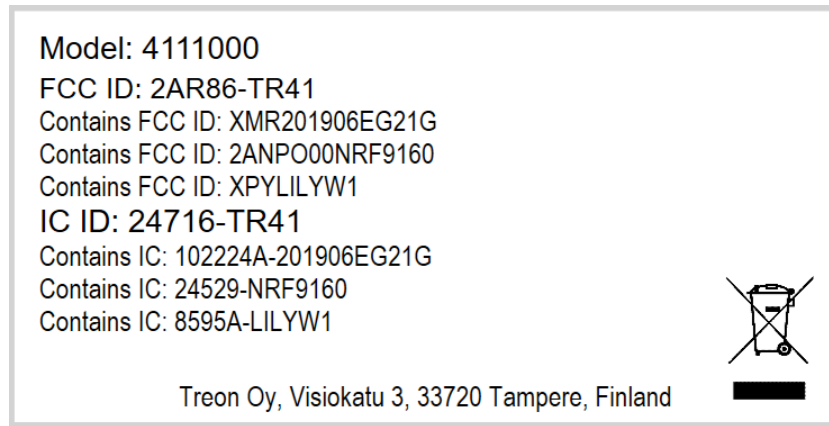
Picture 1. Label example of device 4111000 – Size not in scale. Actual size 2 x 1 inch.
