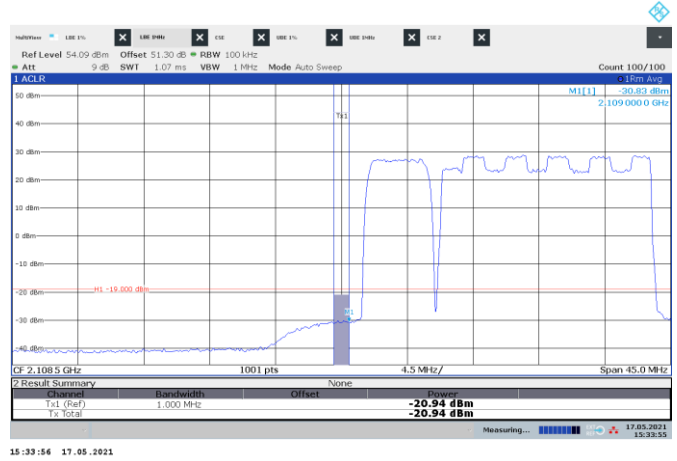
Figure 8.3-190: Conducted emission 1 MHz away from the lower band edge
