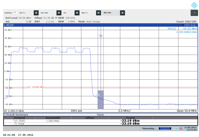
Figure 8.3-128: Conducted emission 1 MHz away from the upper band edge
