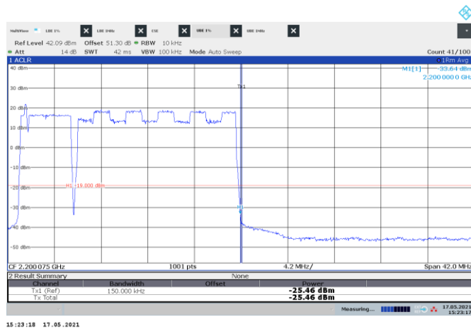
Figure 8.3-175: Conducted emission at the upper band edge
