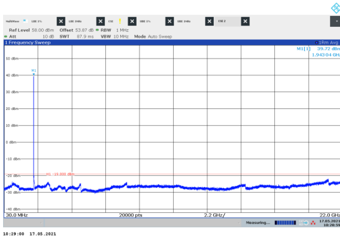
Figure 8.5-40: Conducted spurious emissions of 2xNR 5 MHz contiguous bottom channels, multi-carrier operation
