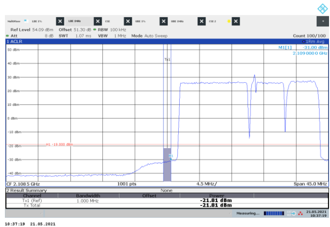
Figure 8.3-170: Conducted emission 1 MHz away from the lower band edge
