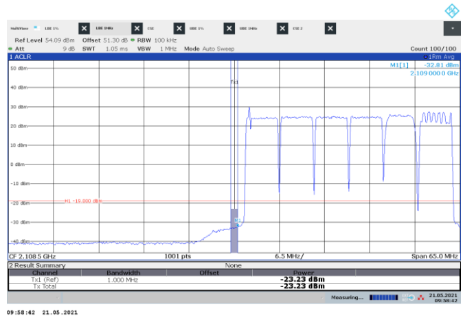
Figure 8.3-150: Conducted emission 1 MHz away from the lower band edge
