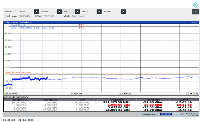
Figure 8.5-49: Conducted spurious emissions of 4xNR 5 MHz contiguous mid channels, multi-carrier operation
