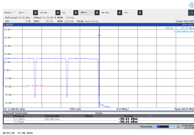
Figure 8.3-139: Conducted emission at the upper band edge
