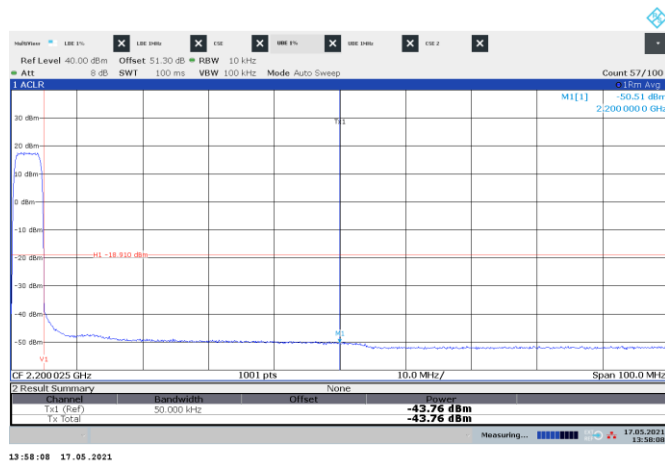
Figure 8.3-147: Conducted emission at the upper band edge
