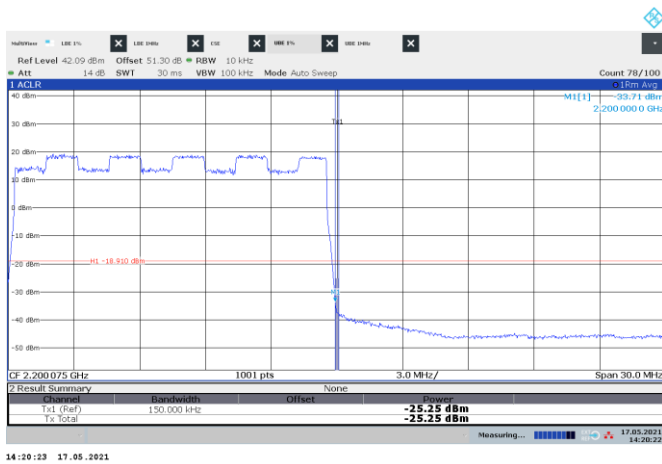
Figure 8.3-127: Conducted emission at the upper band edge
