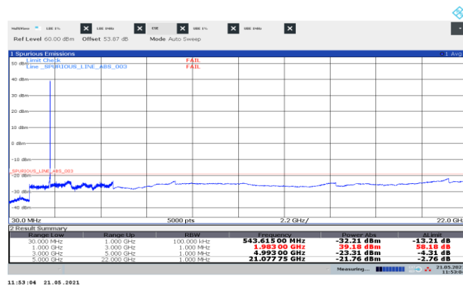
Figure 8.5-25: Conducted spurious emissions of 4xLTE 5 MHz contiguous top channels, multi-carrier operation
