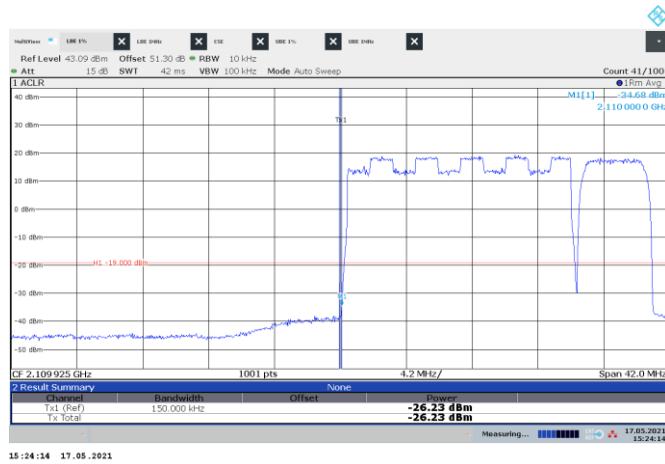
Figure 8.3-177: Conducted emission at the lower band edge
