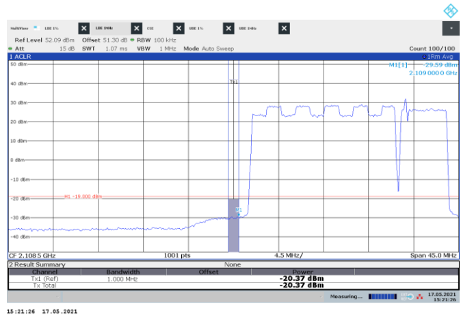
Figure 8.3-174: Conducted emission 1 MHz away from the lower band edge
