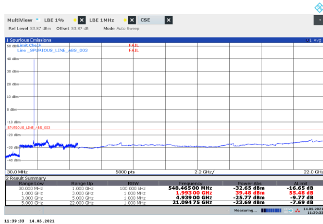
Figure 8.5-3: Conducted spurious emissions of LTE 5 MHz top channel, single carrier operation
