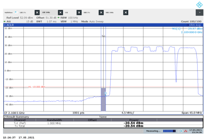
Figure 8.3-178: Conducted emission 1 MHz away from the lower band edge
