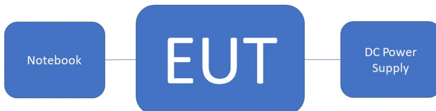
Fig. 2-2 Conducted test set up configuration
