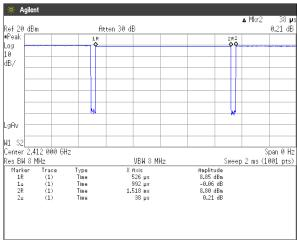
Duty Cycle = Ton / (Ton + Toff) =  $992[\mu s] / (992[\mu s] + 38[\mu s]) = 96.31[\%]$
