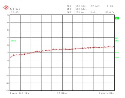
No significant frequencies above the noise floor of the system were found during the preliminary radiated emission test, so no measurements were carried out the open area test site.
