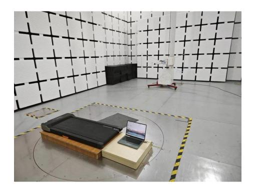
Set-up for Radiated Spurious Emission, Above 1GHz
