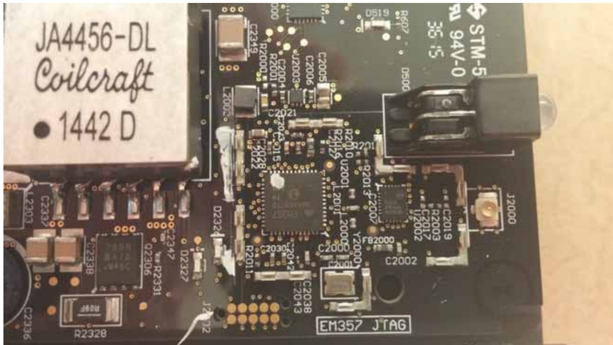
Photograph 10 – View of the Circuitry of the 802.15.4 Transceiver with RF Shield Removed
