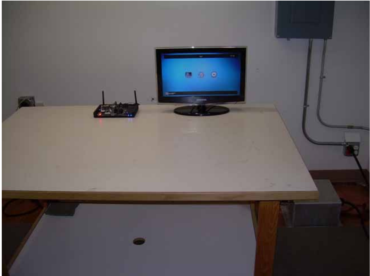
Photograph 3 – Front View of the Conducted Emission Setup
