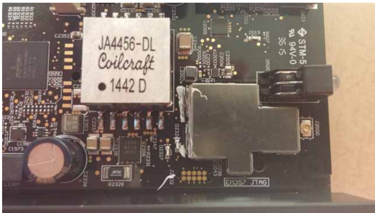
Photograph 9 – View of the 802.15.4 Transceiver Circuitry with RF Shield
