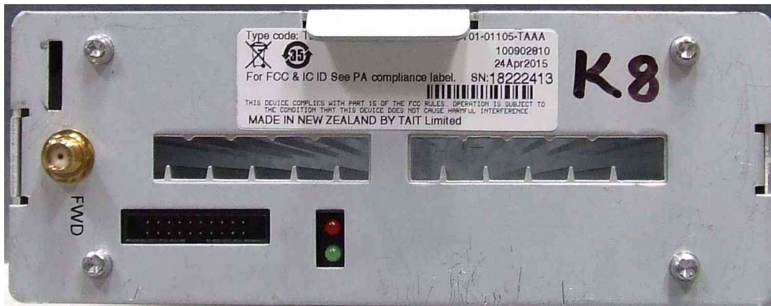
Photograph 02: Reciter module – Front panel
