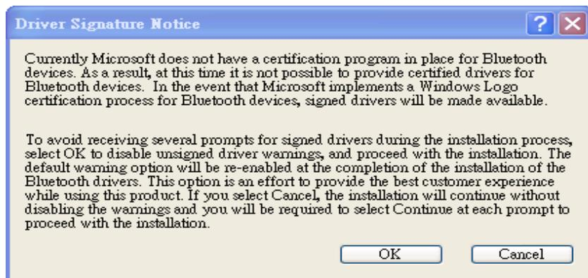
7. After you click “**OK**” button from the Driver Signature Notice dialog box at previous step, the InstallShield Wizard will continue to install WIDCOMM Bluetooth Software.
