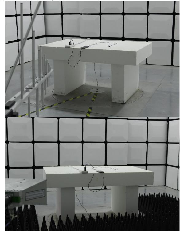
Radiated Emissions Test Setup
