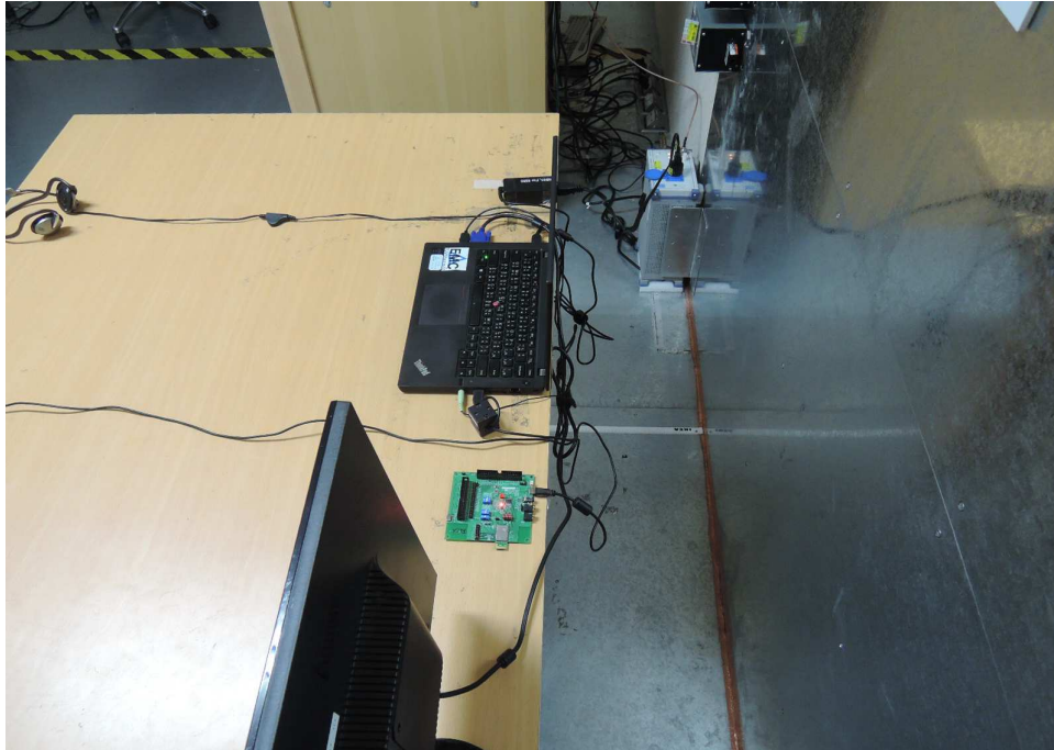
Photograph 5: Set-up for for Mains Conducted testing Back
